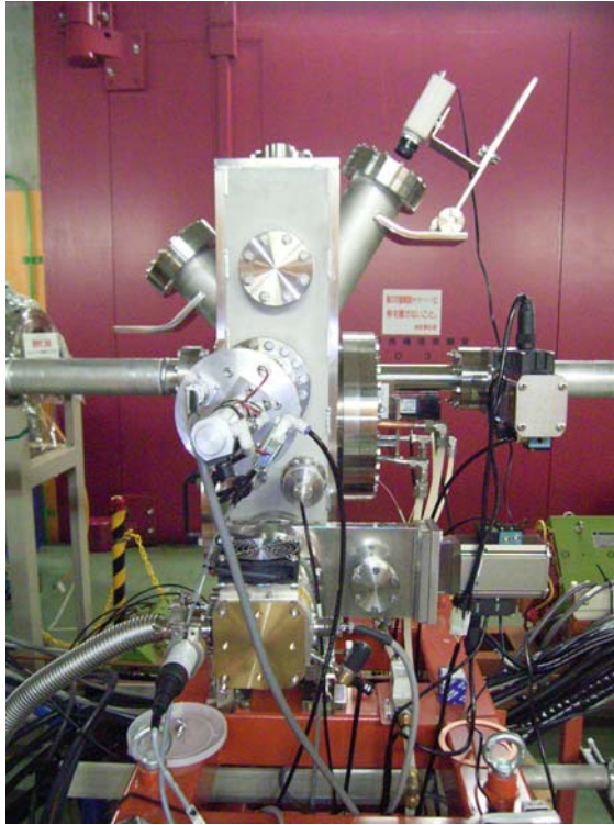
Figure 2. Photograph of the rotating carbon disk stripper.
