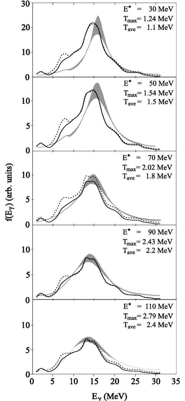
FIG. 2. Experimental (shaded areas) and theoretical divided spectra calculated within the CASCADE model without pairing (dashed curves) and including pairing (solid curves) at various excitation energies.
