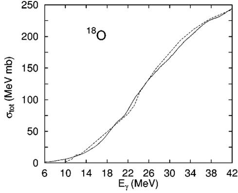
FIG. 2. Running sums of the integrated photoabsorption cross section for  $^{18}\text{O}$ . The solid curve is the result of theoretical calculations within the PDM, while the dashed curve is the experimental result of Ref. [1].
