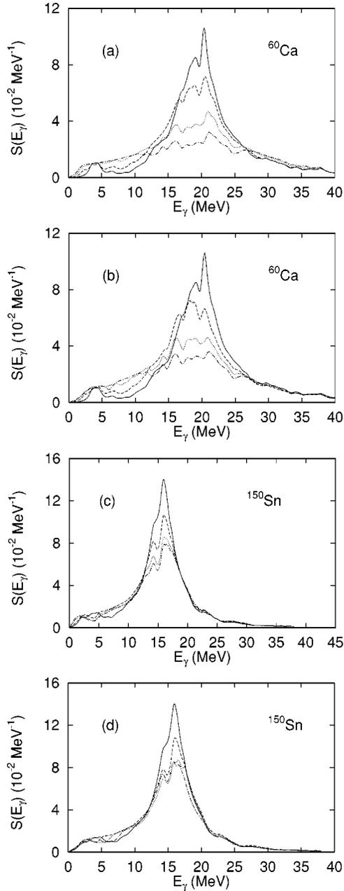
FIG. 5. GDR strength functions in  $^{60}\text{Ca}$  (a),(b) and  $^{150}\text{Sn}$  (c),(d) at several temperatures. The solid, dashed, dotted, and dash-dotted curves correspond to temperatures  $T=0, 1, 2,$  and  $3$  MeV, respectively. (a) and (c): results obtained using the zero-temperature chemical potentials. (b) and (d): results obtained using the temperature-dependent chemical potentials.
